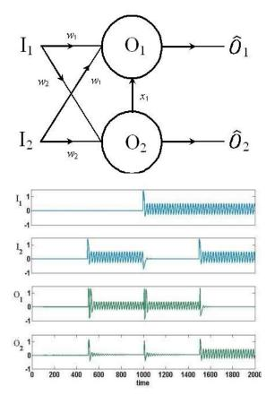
Figure 2: (a) Schematic of a binary oscillator half-adder. (b) Numerical simulation: Time series showing correct logic function of a half-adder. An oscillation corresponds to a 1 in binary and no oscillation is a zero. The sum oscillator  $O_1$  will oscillate if either  $I_1$  or  $I_2$  is active. The carry oscillator  $O_2$  will oscillate if both  $I_1$  and  $I_2$  are active. An inhibitory connection, say  $x_1$ , from  $O_2$  to  $O_1$  suppresses oscillator  $O_1$  if  $O_2$  is active.
