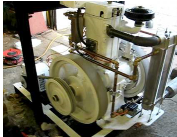
Fig. 2: Photo Image Diesel Engine with Electric Generator
