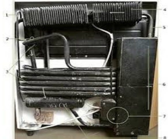
Fig. 3: Photo Image of waste heat absorption system
