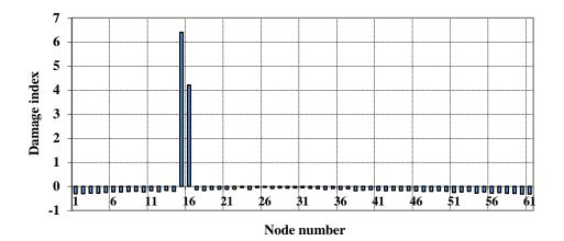
Fig. 7. Damage indices of ULS curvatures of Case 3 of damage
