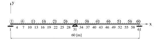
Fig. 1. Geometry of the two-span continuous beam
