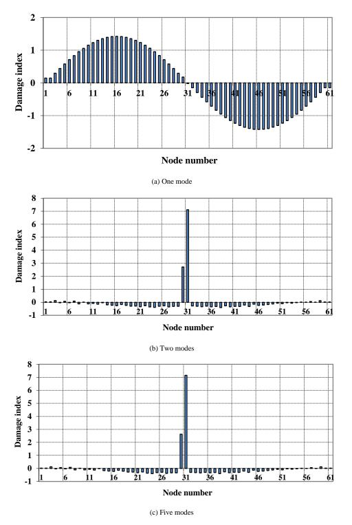
Fig. 3. Damage indices of ULS curvature of Case 4 of damage
