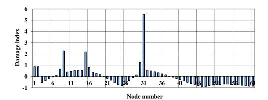
Fig. 8. Damage indices of mode shape curvature of Case 6 of damage
