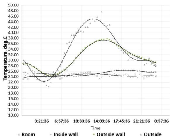
Fig.4d Temperatures distribution for INSULATED wall for 24 hours
