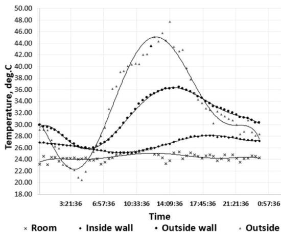
Fig.4a Temperatures distribution for HCBW for 24 hours
