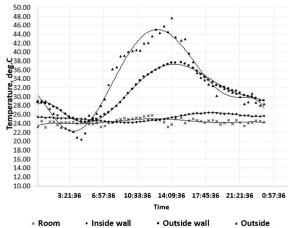
Fig.4c Temperatures distribution for HRBW wall for 24 hours
