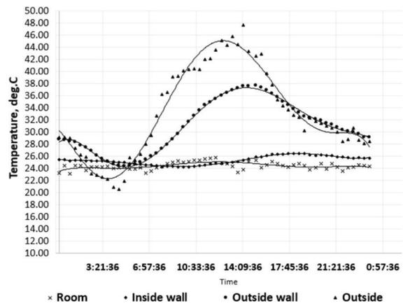
Fig.4b Temperatures distribution for ADOBE wall for 24 hours
