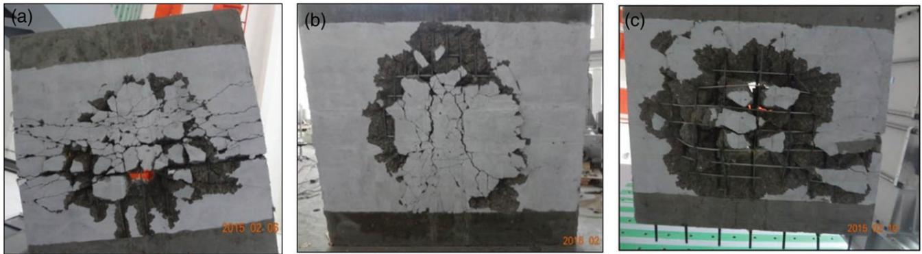
**FIGURE 6** Crack pattern of (a) SS (b) SF and (c) SF0.37P35-0.5 slab
