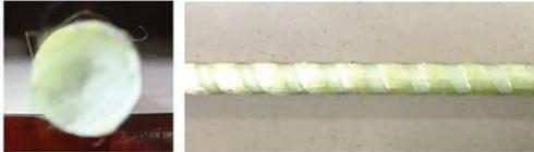
Transversal section and surface of the B/C hybrid bar
