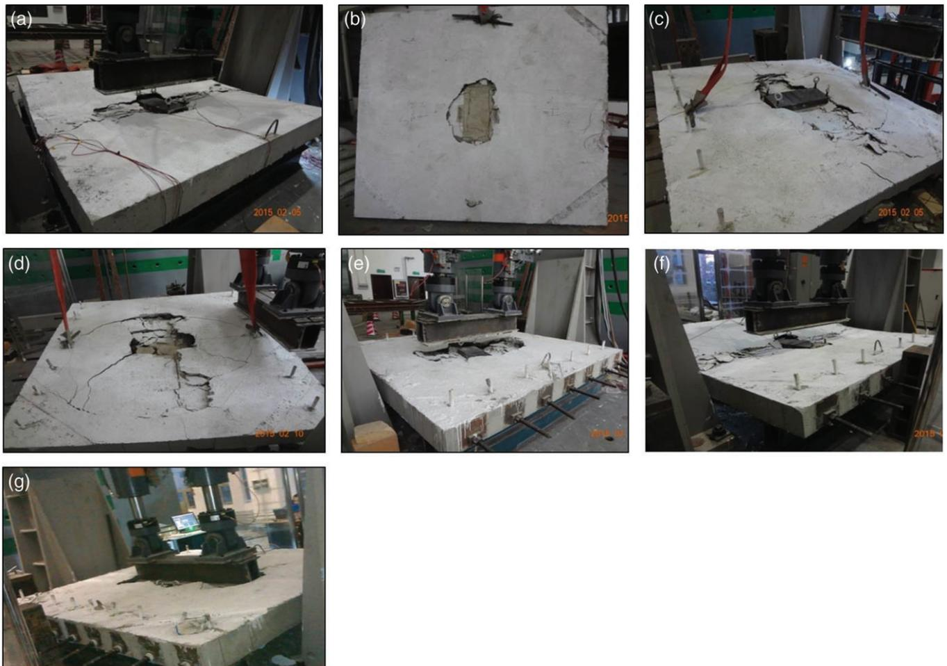
FIGURE 5 Failure modes of (a) SS (b) SF (c) SF0.45P50-0.5 (d) SF0.37P35-0.5 (e) SF0.37P50-0.5 (f) SF0.29P50-0.5 (g) SF0.29P50-0.6
