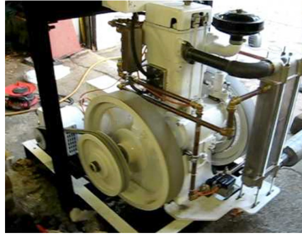
Fig. 2: Photo Image Diesel Engine with Electric Generator
